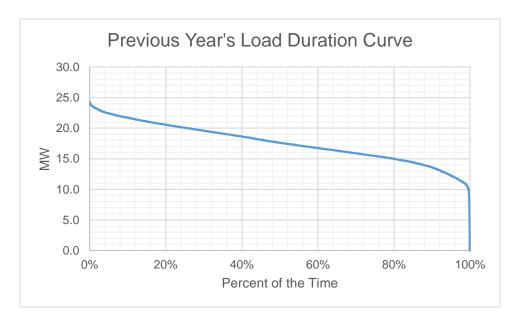
Based on the Load Duration Curve, the minimum load is 7.35 MW and the maximum load is 25.18 MW for the last historical year.
