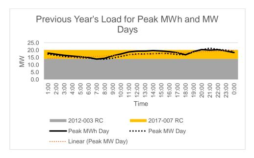
Peak MW occurred on July 6, 2023, and peak daily MWh of 25.18 occurred on the same day at hour 15:00 according to FLECO's load pattern. The available supply is less than the Peak Demand, as demonstrated by the Load Curves.
