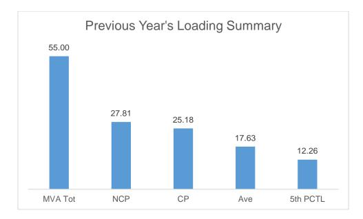
Non-coincident Peak Demand is 27.81 MW, which is approximately 50.56 percent of the substation's total 55 MVA capacity at a power factor of 0.9825. The load factor or the ratio between the average load of 17.63 MW and the non-coincident peak demand is 70 percent. A safe estimate of the true minimum load is the fifth percentile load is 12.26 MW, which is 44.08% of the Non-coincident Peak Demand.
