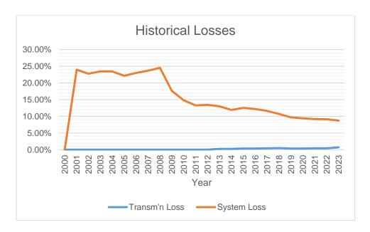
Historically, Transmission Loss varied between 0.23% and 0.43%, whereas System Loss varied between 23.97% and 9.20%. In 2018, transmission loss peaked at 0.46% due to a faulty primary winding of the 5MVA Power Transformer at Lumban 1. System Loss reached a peak of 23.97% in 2001 due to inadequate system loss mitigation strategies.
